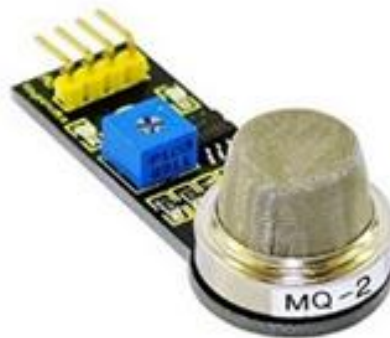
Image 4 MQ-2 Gas Sensor
